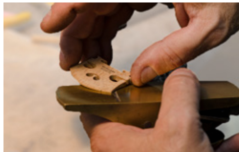
Customising the thickness, lateral shape and curvature.
