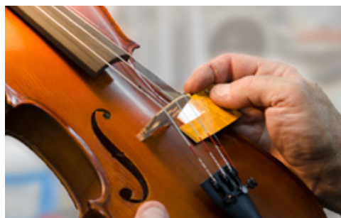
Checking the position of the inserted soundpost.
