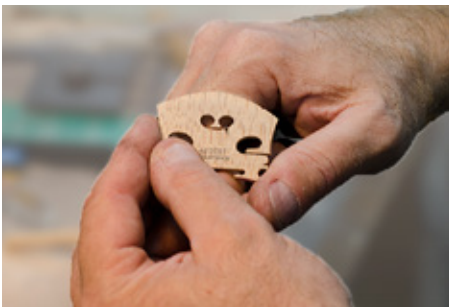
Opening up the 'kidneys,' 'heart' and bridge 'crotch' to increase the liveliness and response of that particular instrument.
