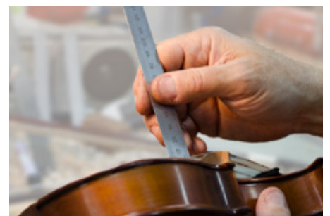
Correct string height from the fingerboard provides both ease of playing and a clear tone.
