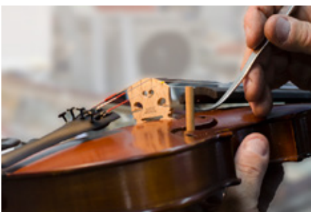
Soundpost must be the correct diameter, the perfect length, and the angle of both ends must match the slope of the belly and back inside the instrument.
